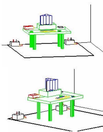
Figure 4. Wooden Table & Bonded LISNs
