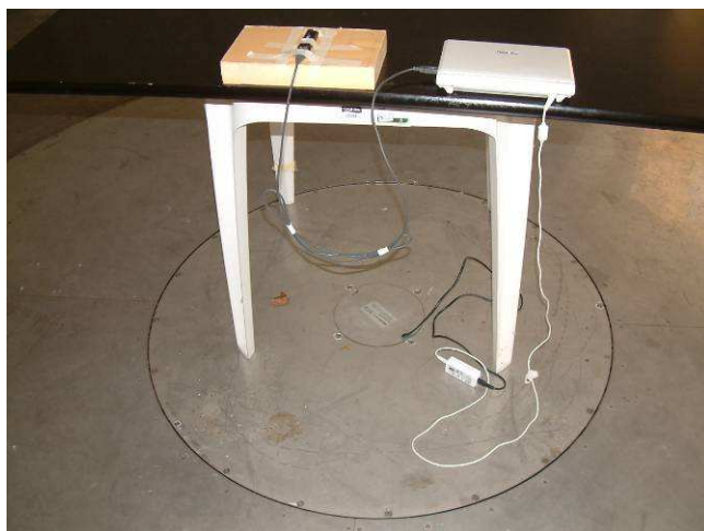
Photo of test setup for Radiated Disturbance
