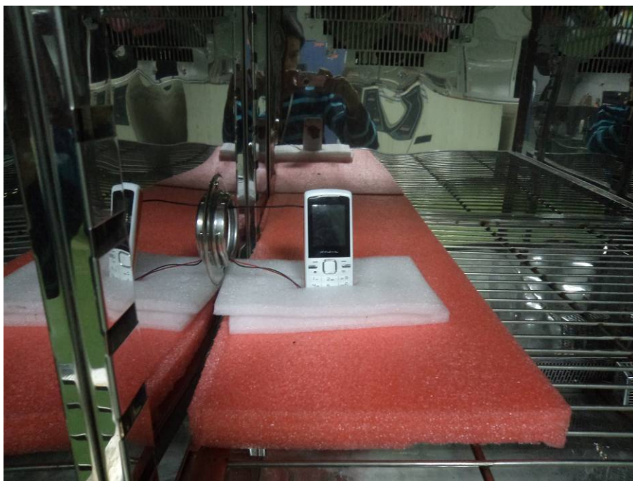
Frequency Stability Test View
