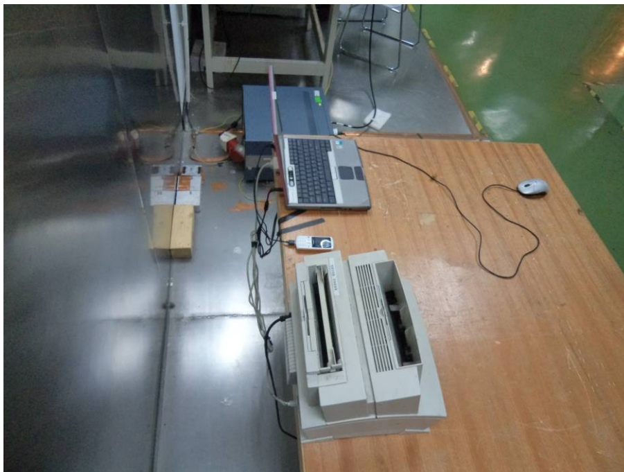
Conducted Emissions - Side View (downloading mode)
