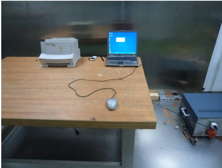
Conducted Emissions - Front View (downloading mode)
