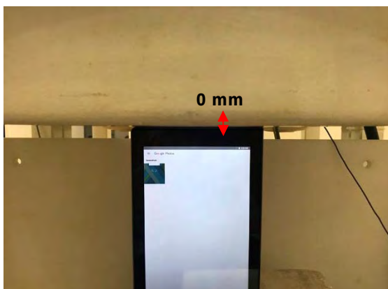
Fig.5 EUT Right side to flat phantom
