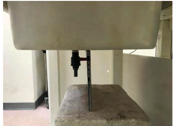
Fig.7 EUT Bottom side to flat phantom
