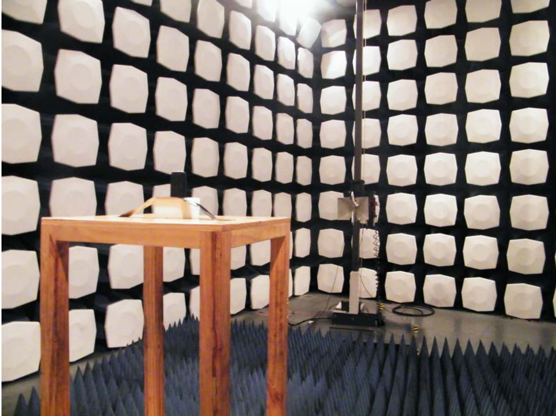
Picture 2: Radiated Spurious Emissions Test setup
