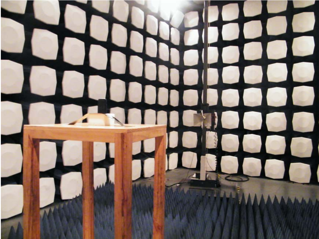
Picture 2: Radiated Spurious Emissions Test setup
