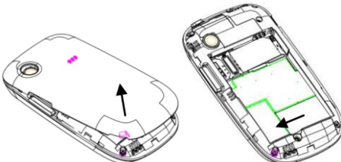
2. Hold the SIM card with the cut corner oriented as shown and slip it into the card holder.
