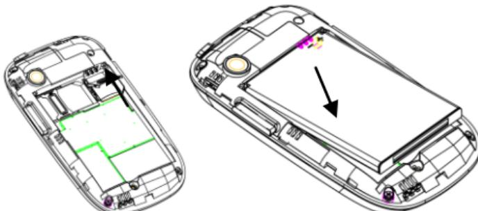
4. Insert the battery by aligning the gold contacts on the battery with the gold contacts in the battery compartment. Gently push down on the battery until it clicks into place.
