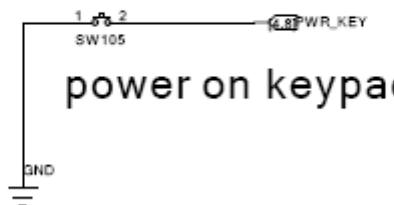
After inserting the battery, VRTC output voltage of 2V, and then the 32.768KHZ crystal start to work. Now press the power on/off switch SW105, then the inner program start initializing. Press the power on/off switch about 2s at normal work status, CPU MT6276 will detect the signal and start the power off program.
