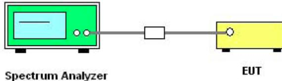
The EUT which is powered by the Battery, is coupled to the Spectrum Analyzer; the RF load attached to the EUT antenna terminal is 50Ω; the path loss as the factor is calibrated to correct the reading. Make the measurement with the spectrum analyzer's resolution bandwidth(RBW) = 100 kHz. In order to make an accurate measurement, set the span greater than RBW.
