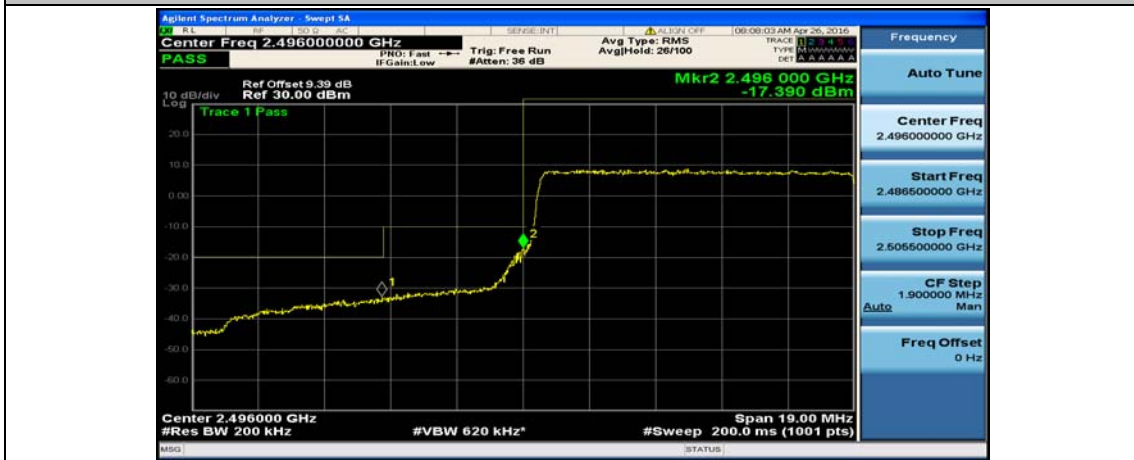
Channel Bandwidth: 10 MHz_LCH_QPSK_50RB#0
