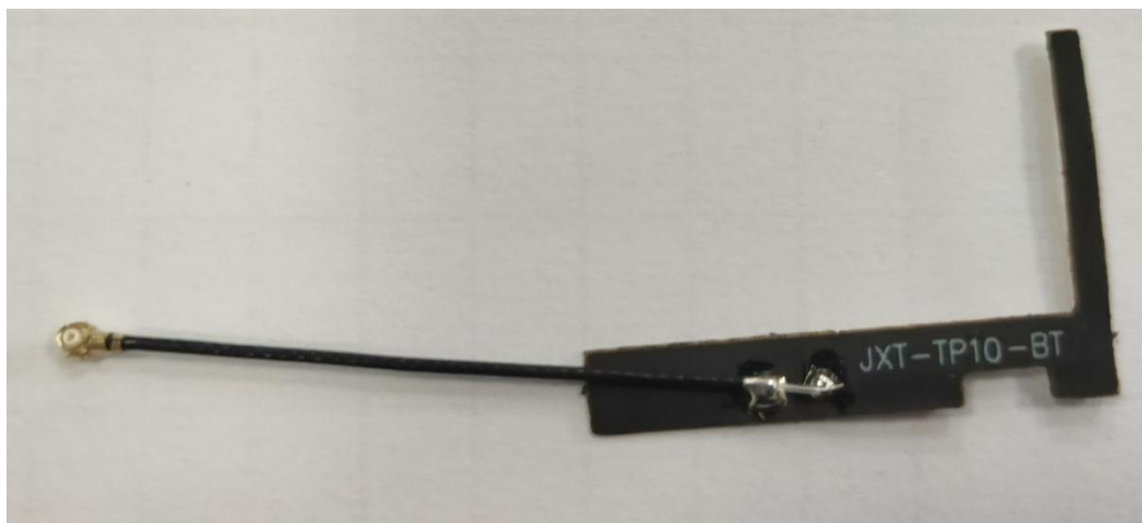
Figure 6: BT Antenna picture
