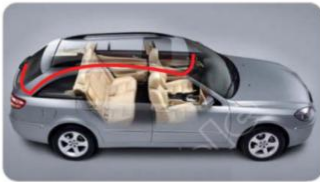
B: Rear camera wiring diagram
