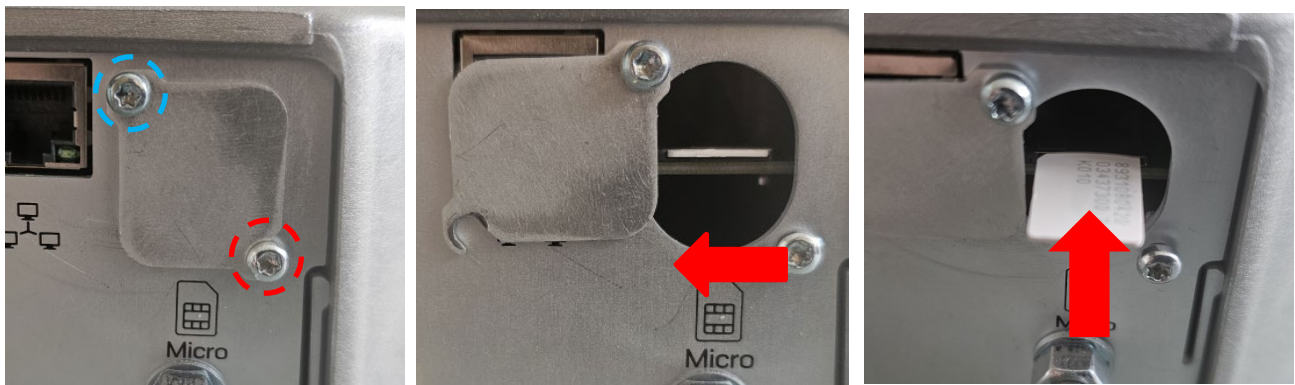
Figure 6 SIM card installation procedure
