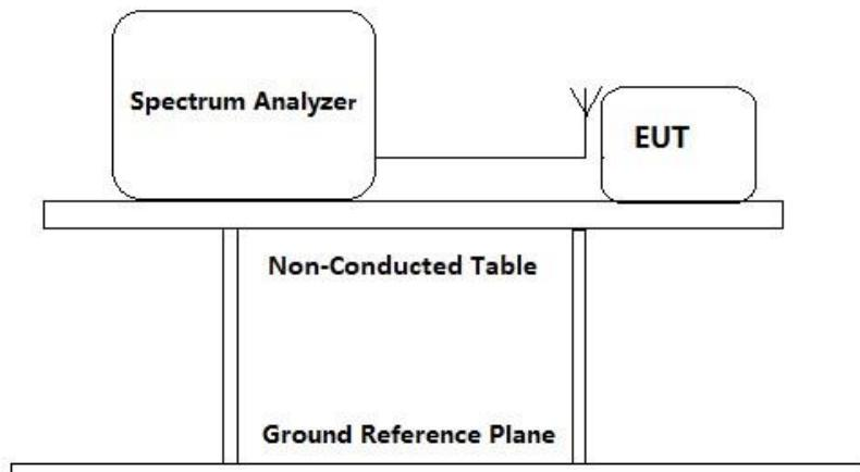
Test Status: Test in transmitting mode at lowest and highest channel.
