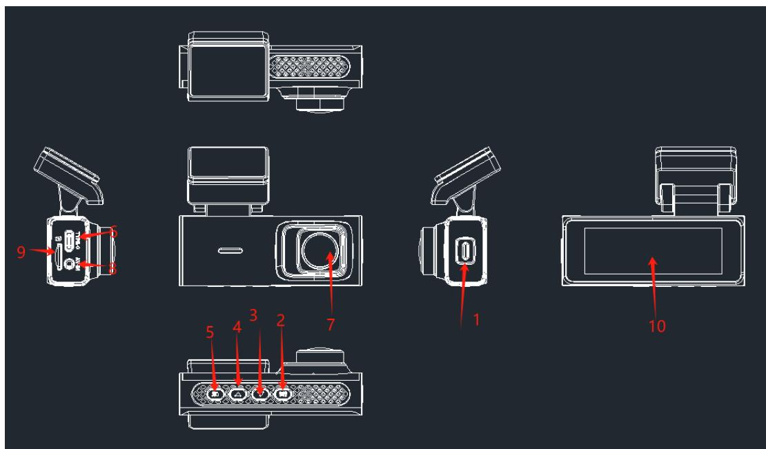
Interface: TP-C interface, AV interface, TF card slot
