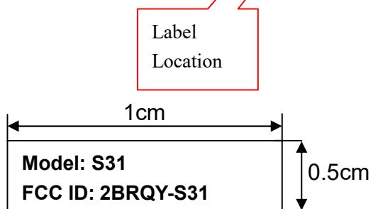
The label is displayed on the EUT by laser engraving.
