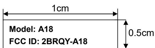
The label is displayed on the EUT by laser engraving.
