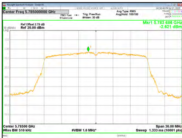
(802.11ac20) PSD plot on channel 157
