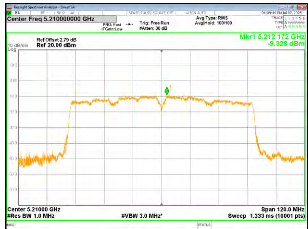
(802.11ac80) PSD plot on channel 42
