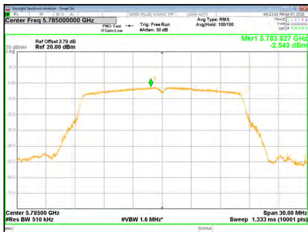
(802.11a) PSD plot on channel 157
