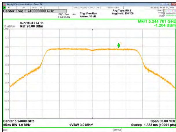
(802.11a) PSD plot on channel 48
