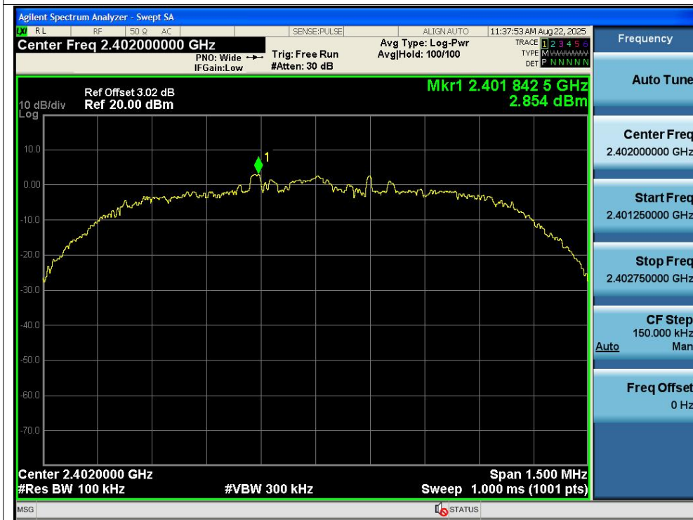
Tx. Spurious NVNT 2-DH5 2402MHz Ant1 Emission
