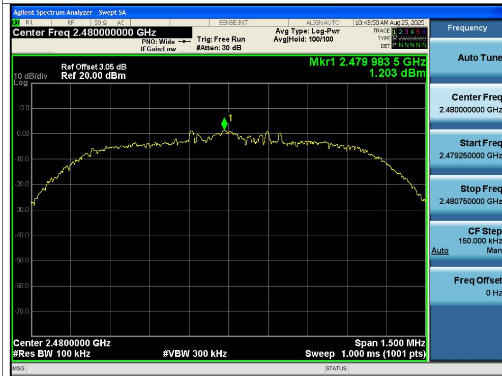
Tx. Spurious NVNT 2-DH5 2480MHz Ant1 Emission
