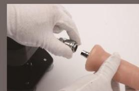
Pull back the head of the self-locking block connector, insert the plug of the appliance into the top of the round hole and loosen it.
