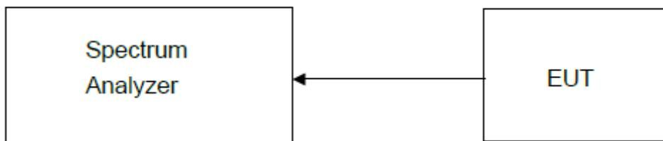
The EUT which is powered by the DC 5V, is connected to the Spectrum Analyzer; the RF load attached to the EUT antenna terminal is 50 Ohm; the path loss as the factor is calibrated to correct the reading. Make the measurement with the spectrum analyzer's resolution bandwidth(RBW) = 100 kHz. In order to make an accurate measurement, set the span greater than RBW.
