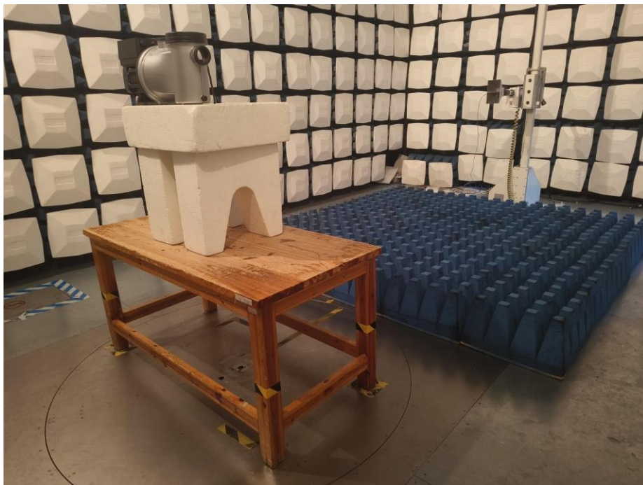
Test Setup For Radiated Emission (Above 1GHz)
