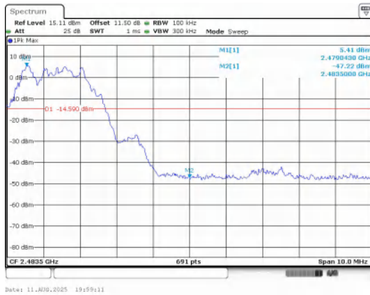
Out Of Band Emission(Right) GFSK_DH5_Channel Hopping
