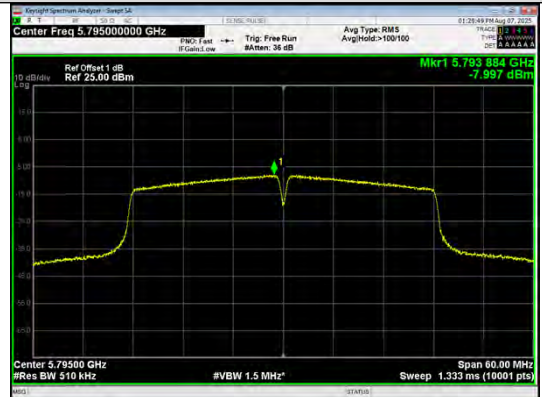
IEEE 802.11n_Channel 159_40MHz_Antenna 0
