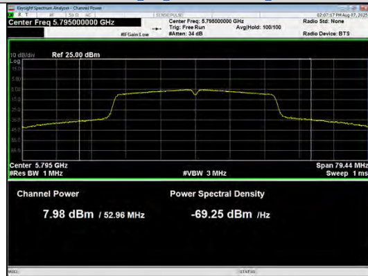
Conducted AVG output power IEEE 802.11ac_40_Channel 159_Antenna 0
