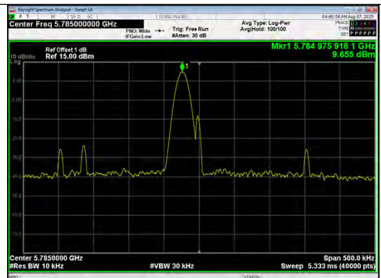
NT/NV_Antenna 0 IEEE 802.11a_Channel 157_20MHz
