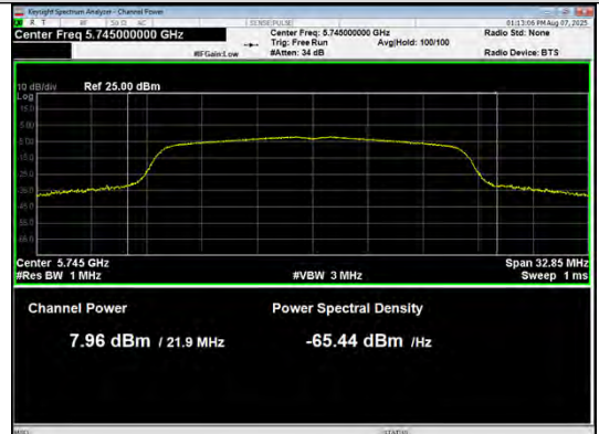
Conducted AVG output power IEEE 802.11a_Channel 157_Antenna 0
