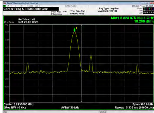
NT/NV_Antenna 0 IEEE 802.11n_Channel 165_20MHz
