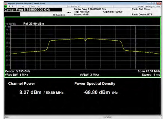
Conducted AVG output power IEEE 802.11ac_40_Channel 151_Antenna 0
