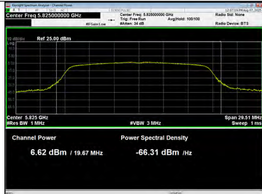
Conducted AVG output power IEEE 802.11a_Channel 149_Antenna 0
