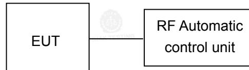
The sample was placed (0.8m below 1GHz, 1.5m above 1GHz) above the ground plane of 3m chamber. Measurements in both horizontal and vertical polarities were performed.
