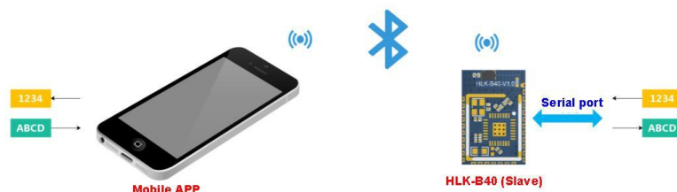
Figure 4 Schematic diagram of one-to-one Bluetooth connection transtransmission function
