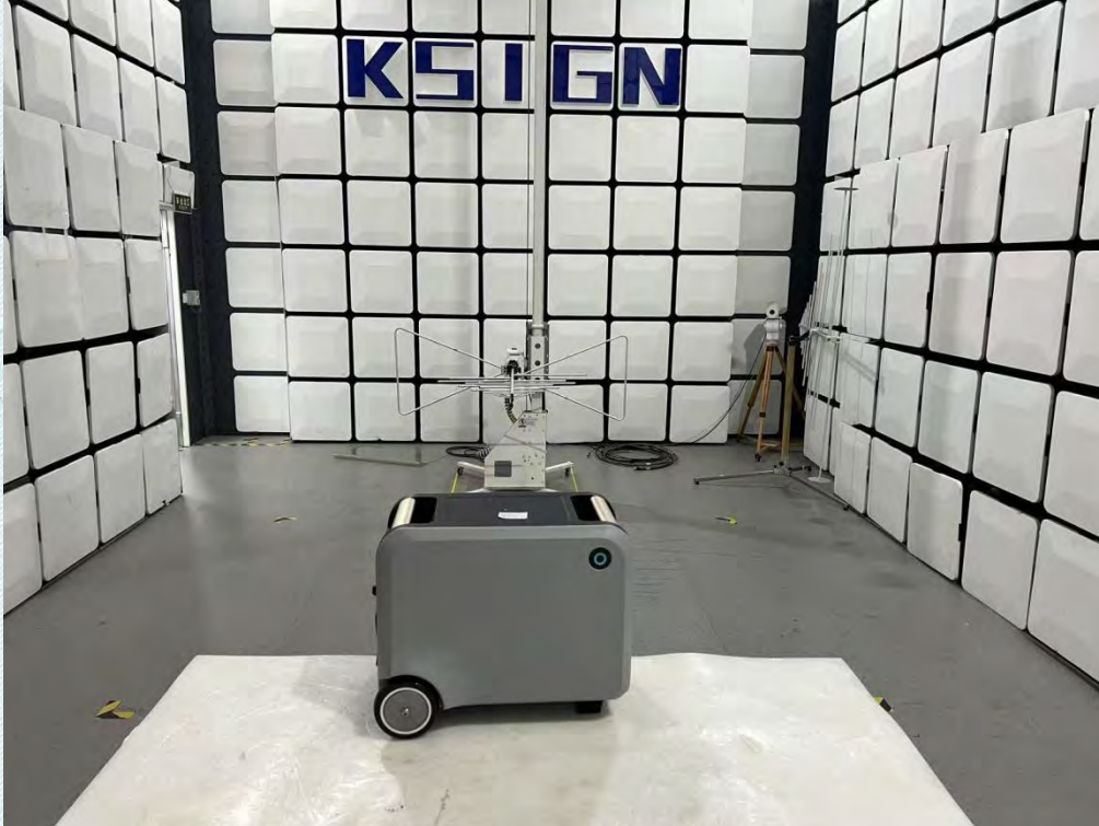
Emissions in frequency bands (below 1GHz)
