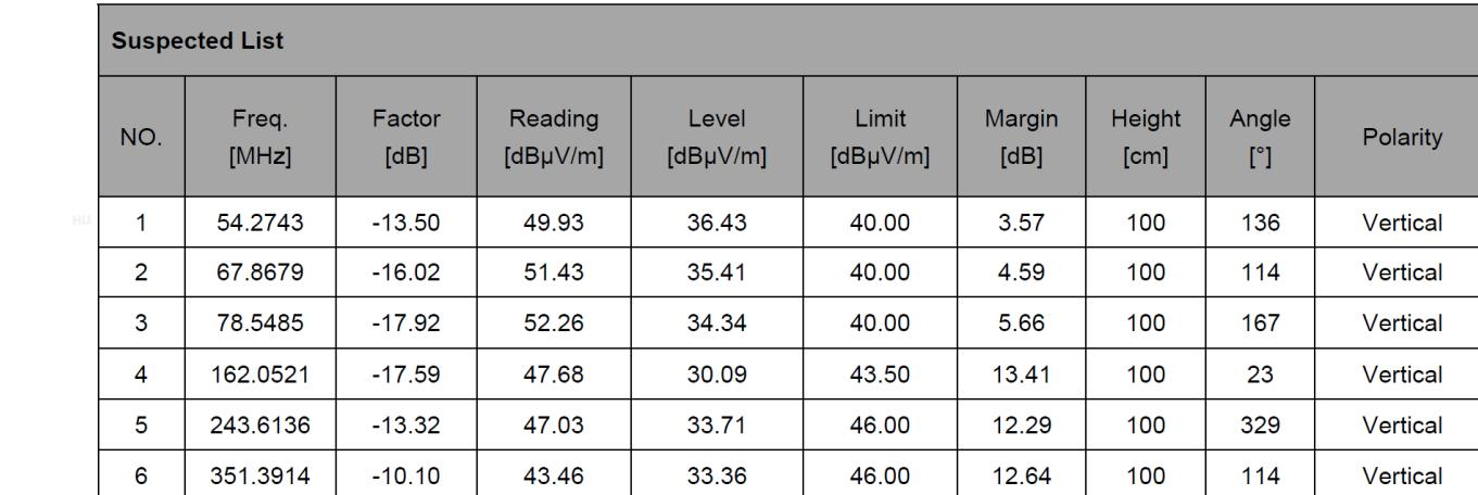
Remark: Factor = Cable loss + Antenna factor + Attenuator – Preamplifier; Level = Reading + Factor; Margin = Limit – Level;
