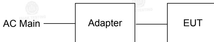
Operation of EUT during 30M-1GHz Radiation testing:
