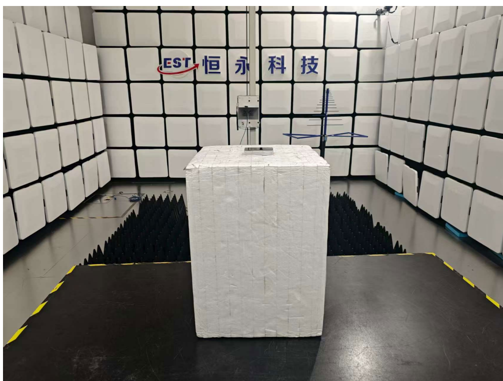
Radiated emission test: Above 1GHz
