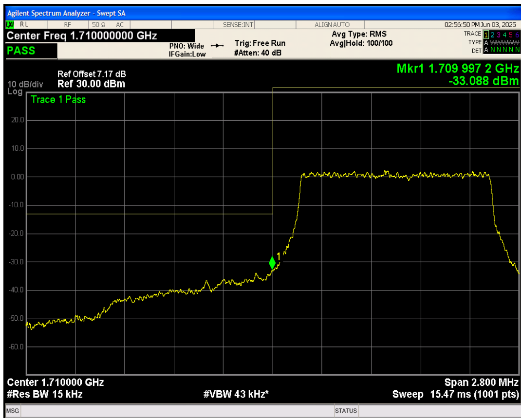
Band66 QAM16 BW=1.4MHz Channel=131979 RB Size=6 Position=#0
