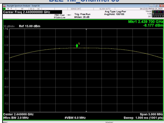
Peak Output Power BLE 2M_Channel 19
