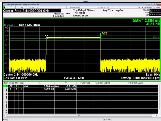
Pulse Width GFSK_DH5
