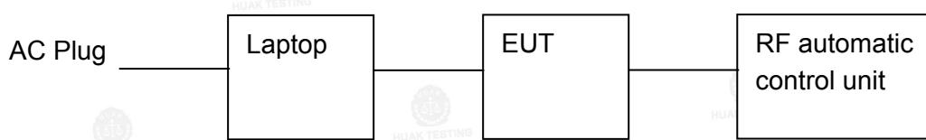
The sample was placed (0.8m below 1GHz, 1.5m above 1GHz) above the ground plane of 3m chamber. Measurements in both horizontal and vertical polarities were performed.
