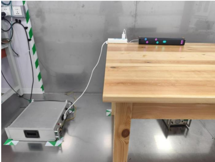
Conducted Emission at AC power line
