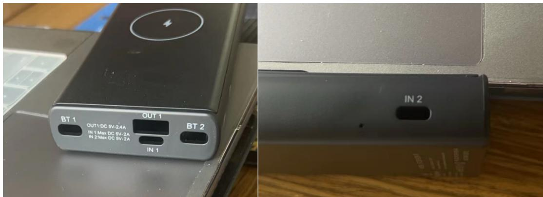
BT2: Press and hold for 2 seconds to power the device on/off. It can also charge devices like phones and wireless charging.
