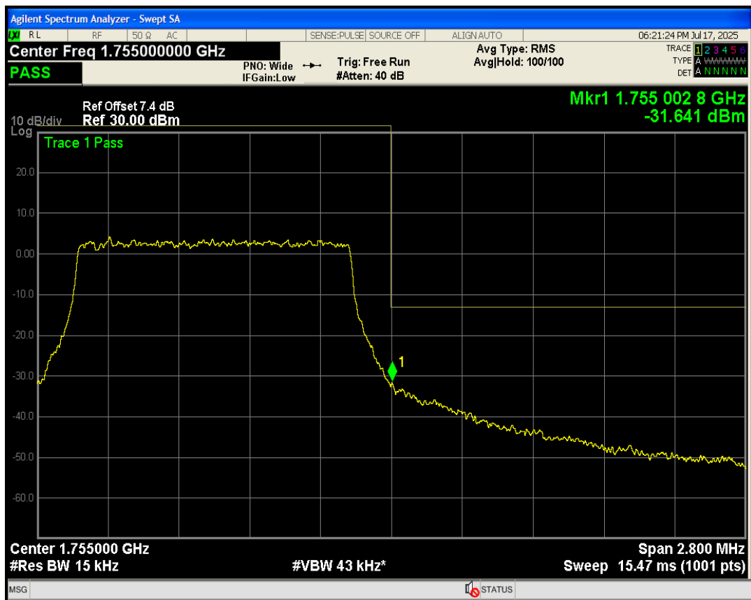
Band4 QAM16 BW=1.4MHz Channel=20393 RB Size=6 Position=#0
