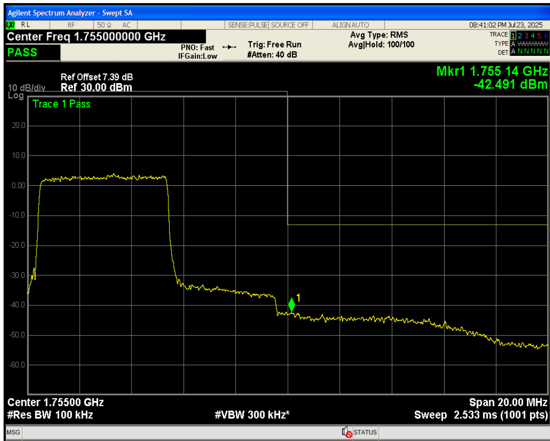
Band4 QAM16 BW=15MHz Channel=20025 RB Size=27 Position=#0
