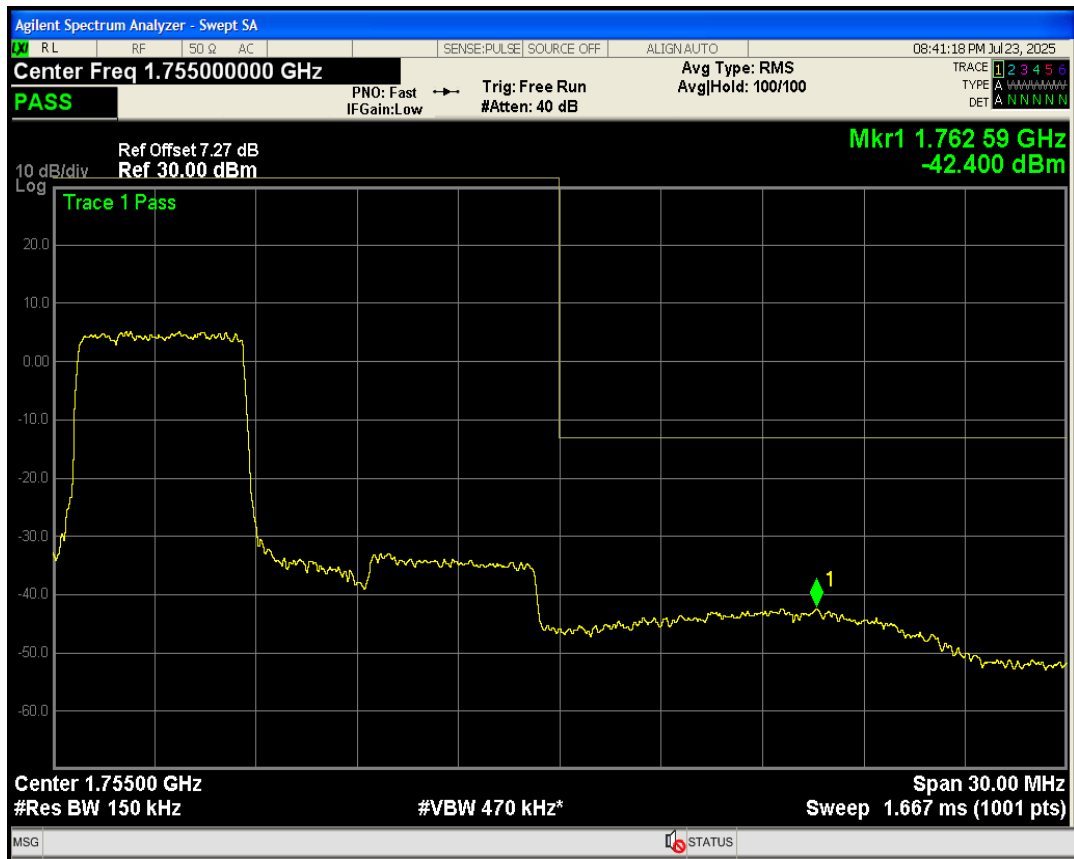
Band4 QPSK BW=20MHz Channel=20050 RB Size=100 Position=#0
