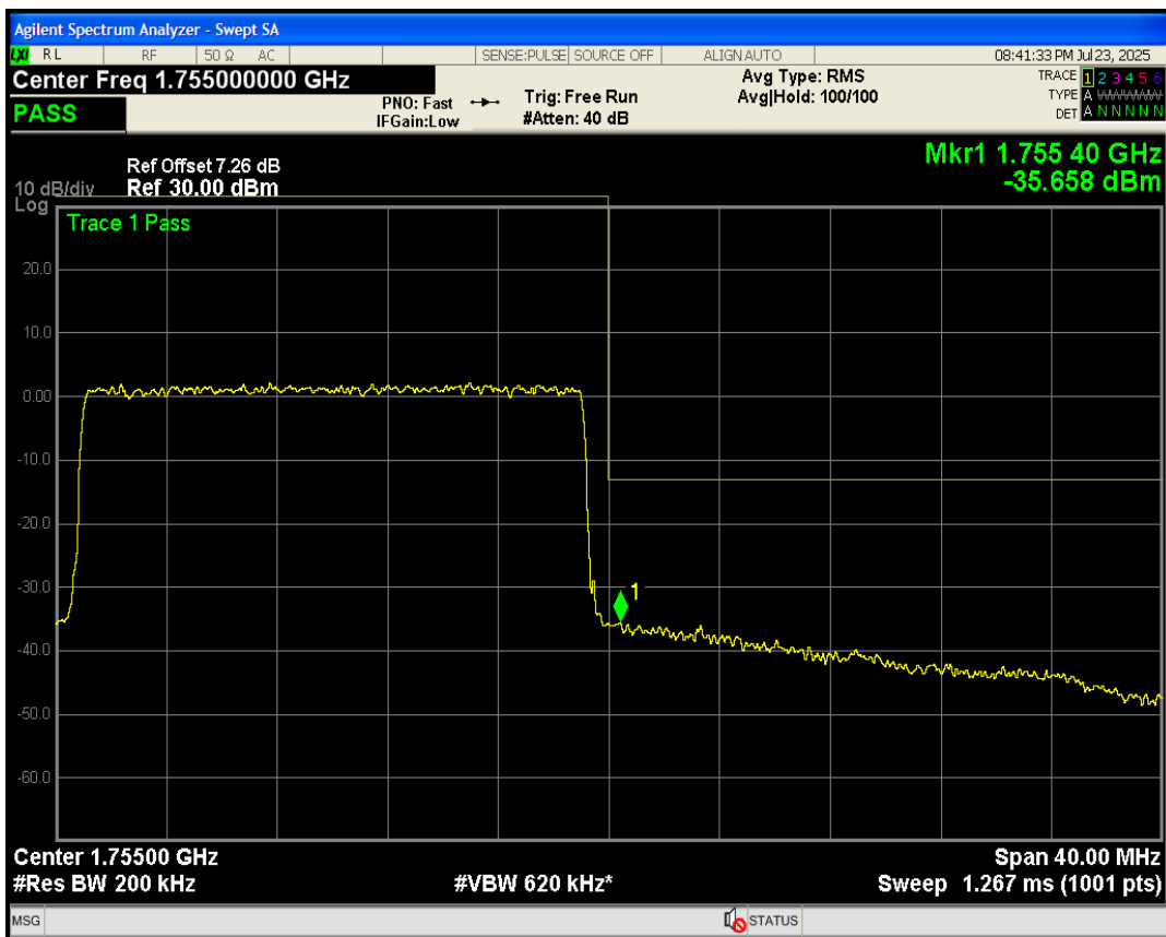
Band4 QAM16 BW=20MHz Channel=20300 RB Size=27 Position=#0
