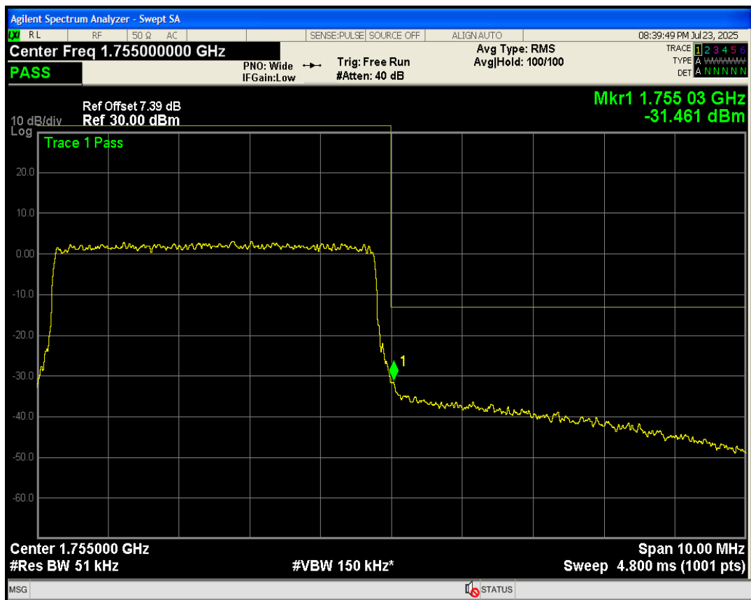
Band4 QAM16 BW=5MHz Channel=20375 RB Size=25 Position=#0
