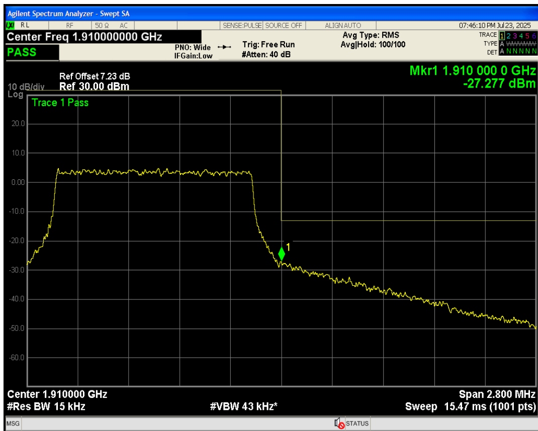
Band2 QPSK BW=1.4MHz Channel=19193 RB Size=6 Position=#0
