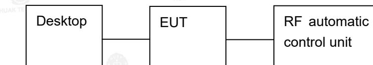
The sample was placed (0.8m below 1GHz, 1.5m above 1GHz) above the ground plane of 3m chamber. Measurements in both horizontal and vertical polarities were performed.
