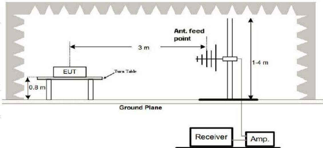
The radiated emission tests were performed in the 3 meters chamber test site, using the setup accordance with the ANSI C63.10-2013. The specification used was the FCC 15.209 and FCC 15.205 limits.
