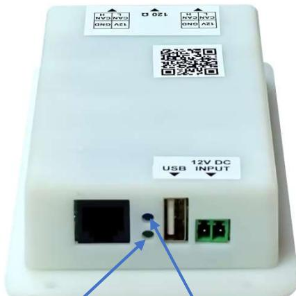
The green LED indicator is solid when the module is powered on
