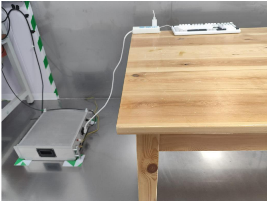
Conducted Emission at AC power line
