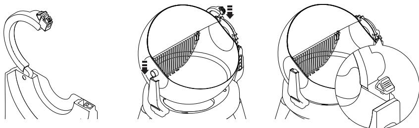
Note: It is necessary to repeatedly confirm the locking condition of the fixed gate to avoid the litter drum from slipping out.
