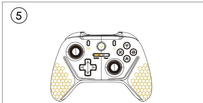
To gain the authority of physical controller, hold the Switch button for 2-3s to gain the authority. Once Yarbo gains authority, you can control the yarbo now.
