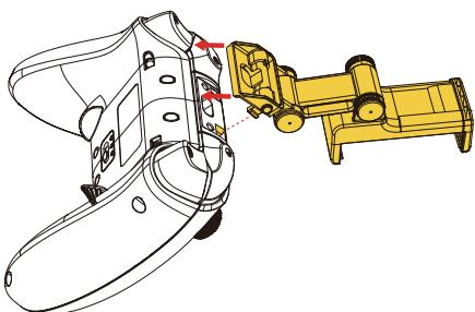
Locate the Physical Controller Holder provided in the Yarbo Core package and locate the side button on the Holder.
