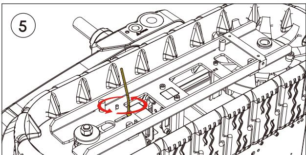
Unscrew the bolt shown in the picture using Allen Key#4
