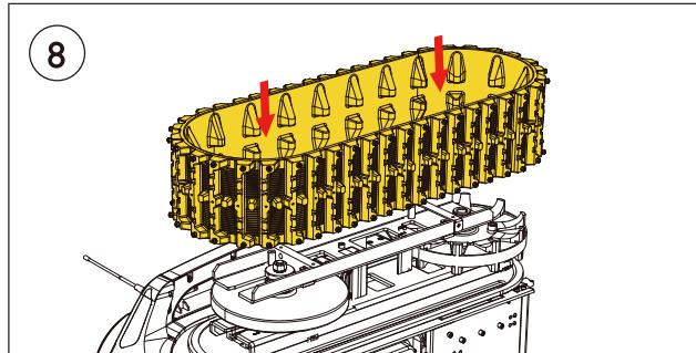
Locate the Snow Track provided in the package and install the Snow Track. Please ensure the track direction is correct as shown in the picture.
