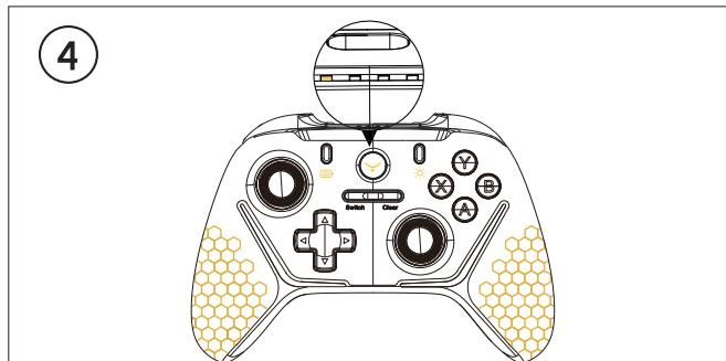
Observe the LED light on the top of Yarbo Controller. If the left yellow light is on steadily, it indicates that connected with the phone.
