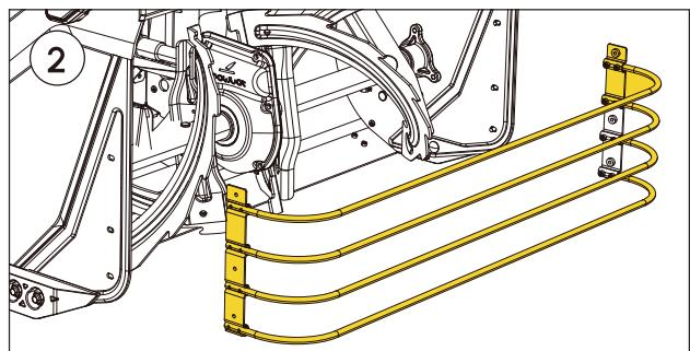
**Remove** the protection fence and safely preserve the bolts and fence.
