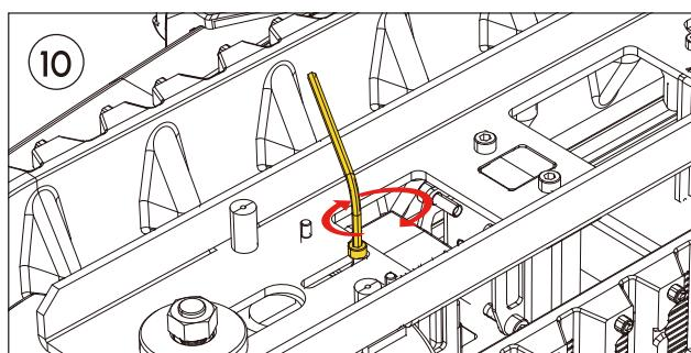
Tighten the bolt using Allen Key#4
