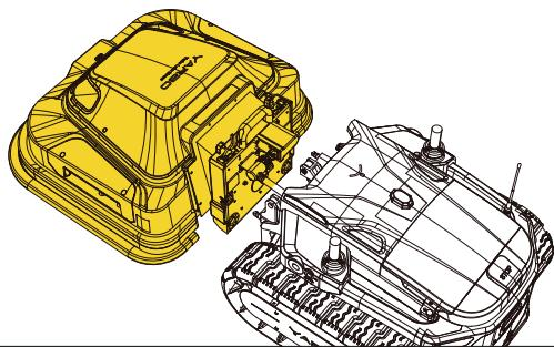
Please remove the module in the front for better adjusting the track.
