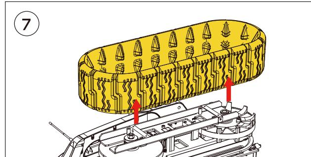
Tap both ends of the track and carefully detach the track from the Yarbo Core. If it is still too hard to detach the track, please repeat step 4 and step 5.
