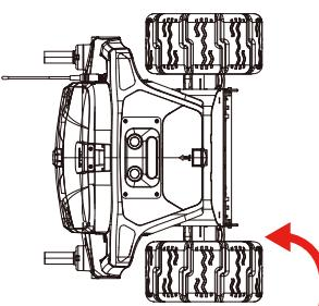
Rotate the Yarbo Core to a vertical position on its side.
