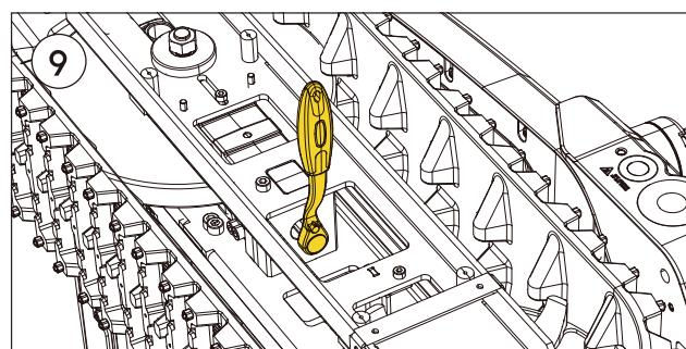
Locate the Track Wrench and tighten the bolt.
