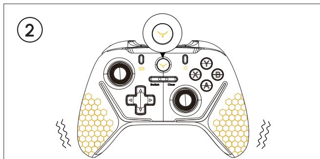
Press and hold the Yarbo Logo Button for approximately 5 seconds to turn on the physical controller and initiate the pairing mode.
