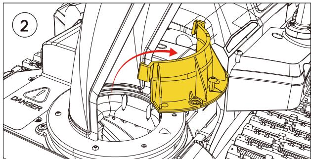
**Remove** the Snow Plume Diverter.
