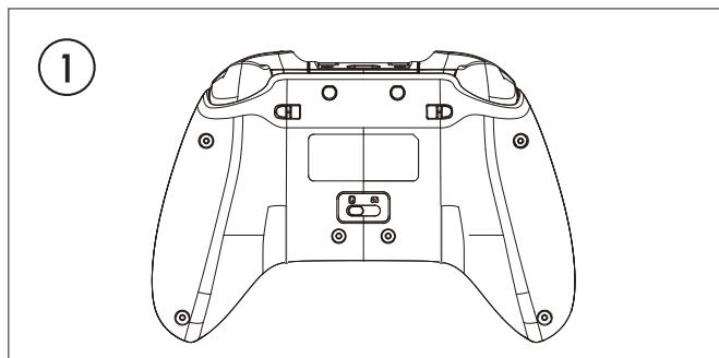
Make sure that the slide switch is slid to the left side.
