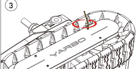
Remove the Side Panel by unscrewing the four bolts shown in the picture using Allen Key#2.
