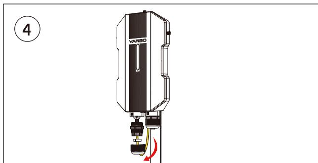
Thread the ethernet cable through the gland and its cover. Locate the opening of the black rubber plug and snap it onto the ethernet cable.
