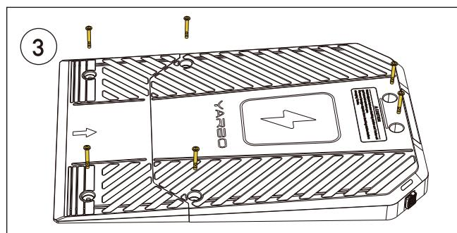
**Place** the Docking Station on the desired location. Secure the Docking Station by suitable methods. For soil/grass surface, use grass pegs. For concrete/brick surfaces, use expansion bolts. Grass pegs and expansion bolts are provided in the package
