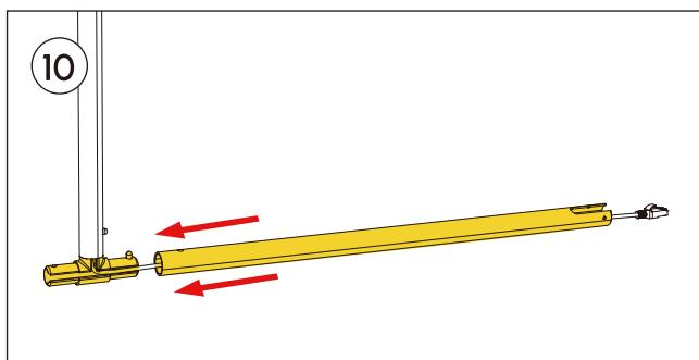
Press the round button on the T-joint and align it with the hole in the standard pole to connect two parts and secure the connection.
