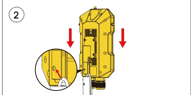
Connect the Data Center to the extension pole (press the small button on the data center and aligning this button to the hole in the pole). Pull out a small section of the cable to ensure it can be reached and connected to the ethernet port.
