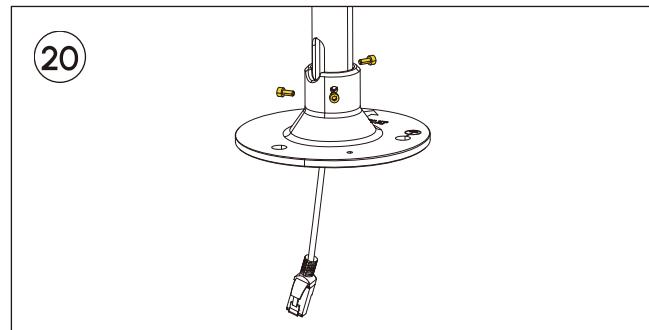
Screw in three connection bolts for pole to stabilize the mount and standard pole.
