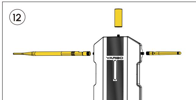
Locate the three antennas provided in the YARBO Core box and securely tighten them.
