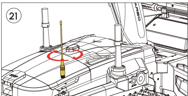
**Locate** the Halow Antenna for Rover provided in the package and install the antenna by screwing it into the place shown in the picture.
