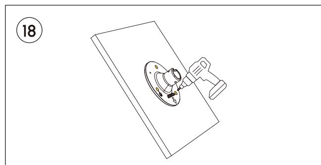
Position the mount on the roof and mark the locations for four holes (5/16" or 8mm). Drill the holes, ensuring that the center hole is drilled to an adequate depth to allow the ethernet cable to be threaded into the house for router connection.
