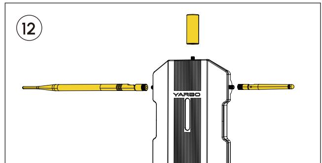
Locate the three antennas provided in the Yarbo Core box and securely tighten them.
