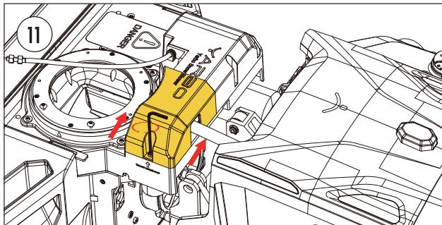
**Place** the protection cover back to its original position by putting it down on the track and sliding it to the end. Screw the connection screw to tighten the cover using Allen Key #2.
