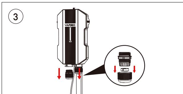
Carefully unscrew the entire gland set located on the WAN port of the Data Center. Remove the gland cover and push out the black rubber plug.
