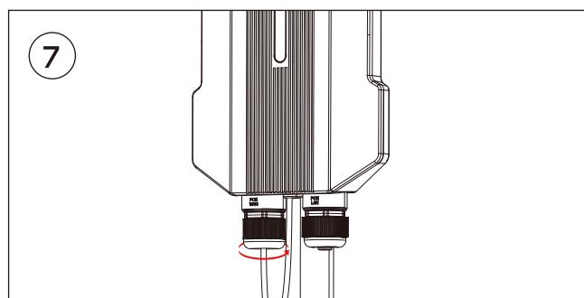
Screw and tighten the cover of the gland.
