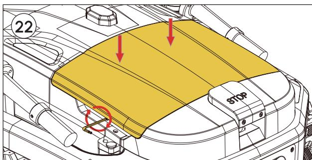
**Place** the battery cover back in place and screw the Anti-theft Bolts on both sides using **Battery Cover Wrench** provided in the package.
