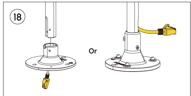
Thread the ethernet cable through the middle hole of the mount, or pull out the Ethernet cable through the opening or gap in the pole carefully.
