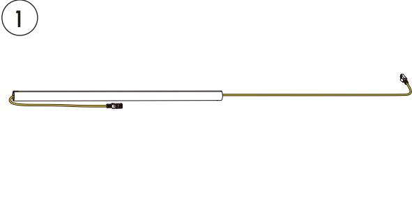
Locate the ethernet cable and extension pole provided in the Yarbo Core box. Thread the ethernet cable through the extension pole.
