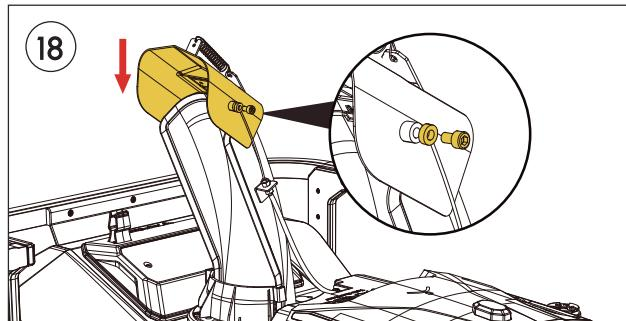
**Unscrew** the bolt shown in the picture. Press down the deflector on the chute. Insert the bolt through the ring at the end of the cable, and screw the bolt back in place using Allen Key #4.
