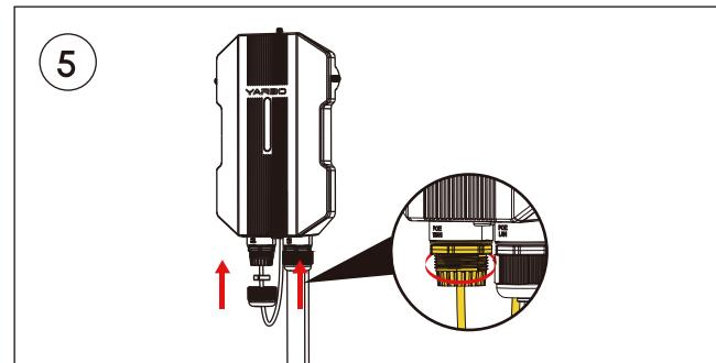
Connect the ethernet cable to the WAN port and tighten the gland by screwing it in.
