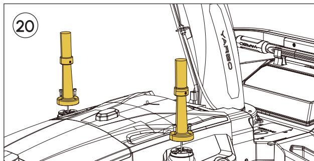
**Straighten** the RTK antennas and locate six Low RTK Antenna Mount Bolts provided in the package. **Screw** the six bolts using Allen Key #2.
