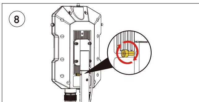
Screw one connection bolt to fasten the connection part between the Data Center and the extension pole.
