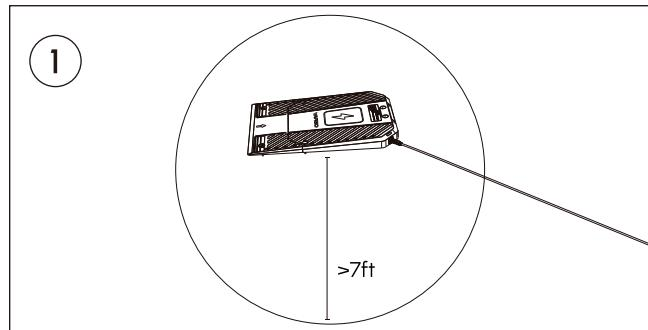
Ensure the installation location for the Docking Station has at least **7 feet** of clearance in all directions. Before proceeding, make sure you have already initialized Yarbo using the Yarbo App.
