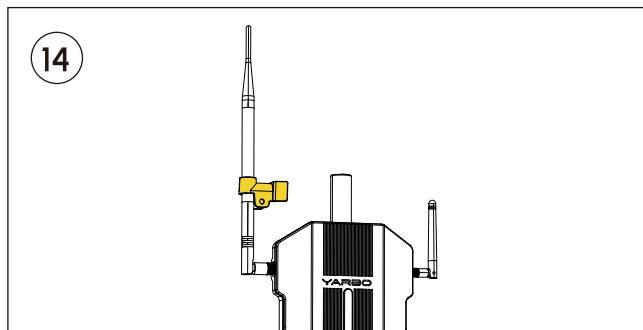
Locate the Halow Antenna Clips through the Halow Antenna.
