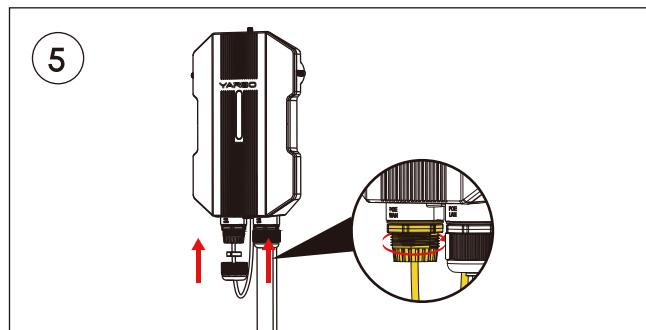
Connect the ethernet cable to the WAN port and tighten the gland by screwing it in.
