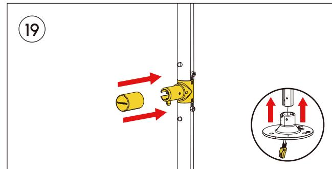
Attach the cap securely to the side of the T-joint.
