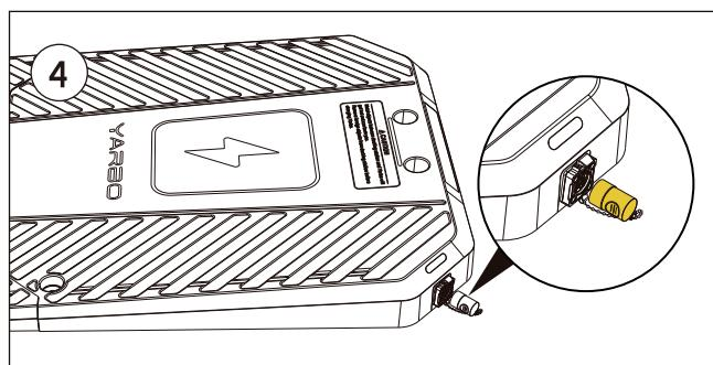
Press the snap and remove the cover
