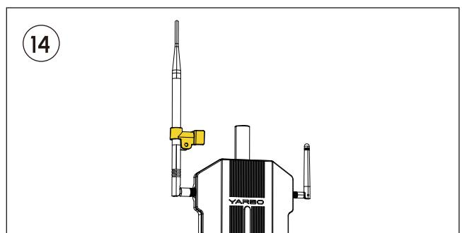
Locate the Halow Antenna Clip through the Halow Antenna.
