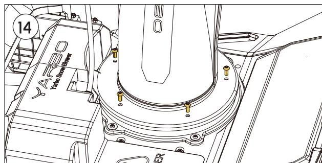
**Locate** the four Snow Chute Connection Bolts and the Snow Chute in the package. **Tighten** the **4 smaller bolts** to fasten the Snow Chute using Allen Key #1.
