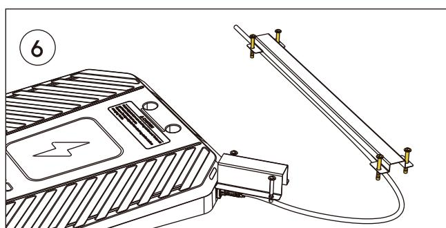
Place the Short Cable Ramp near the port and place the Long Cable Ramp on the Power Cable. Secure the Cable Ramp by suitable methods.
