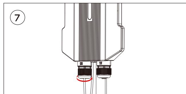
Screw and tighten the cover of the gland.
