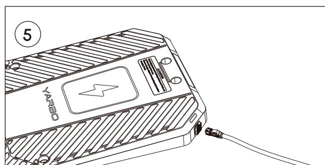
Connect the Power Cable to the port in the docking station
