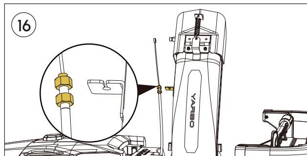
**Locate** the cable shown in the picture. Loosen the **top one** of the two nuts in the middle with Simple Wrench.
