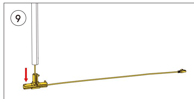
Press the cable into the crevice of a T-joint as shown in the picture. Connect the extension pole to the T-joint by pressing the round button on the T-joint and align this button with the hole in the extension pole.
