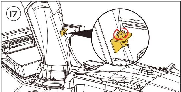
**Place** the cable in the open loop and screw the top nut with Simple Wrench to tighten the cable.
