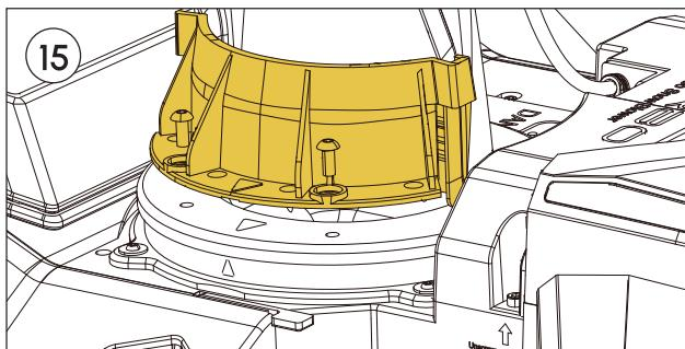
**Locate** the Snow Plume Diverter and the **two** Snow Plume Diverter Connection Bolts. **Tighten** the bolts to fasten the Snow Plume Diverter using Allen Key #2.
