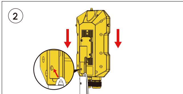
Connect the Data Center to the extension pole (press the small button on the data center and aligning this button to the hole in the pole). Pull out a small section of the cable to ensure it can be reached and connected to the ethernet port.
