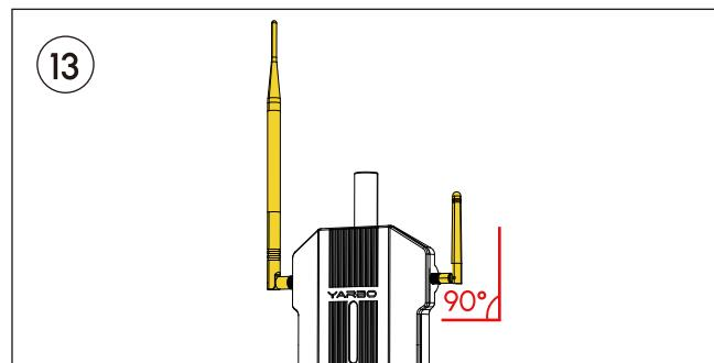
Fold the Halow Antenna and Bluetooth Antenna at a 90-degree angle, directing them upwards towards the sky.
