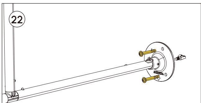
Secure the mount by fastening the three connection bolts. Use wood screws for wooden surfaces, expansion bolts for hard surfaces like concrete or walls and grass pegs for lawns.
