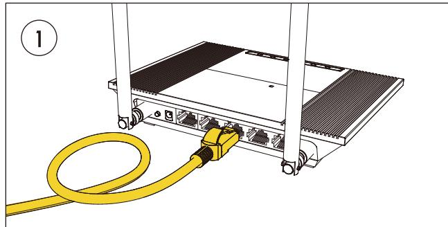
Locate the 2-meter long ethernet cable and the POE power adapter provided in the Yarbo Core Box and connect one side of the ethernet cable to the router.
