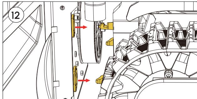
**Locate** the four shafts and holes. Do not push the two parts together right now.
