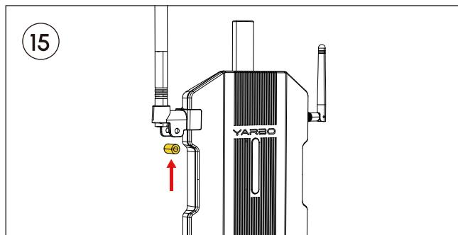
Move the Halow Antenna Clips to the bottom of the Halow Antenna and snap the Data Center. Then put on the Clip bushing.
