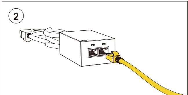
Connect the other side of the ethernet cable to the LAN port of POE power adapter.
