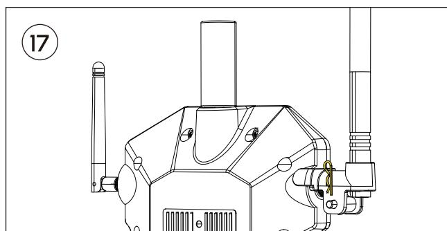
Pass the R-clip through the holes in the Clevis Pin, making sure the Clevis Pin are secure.
