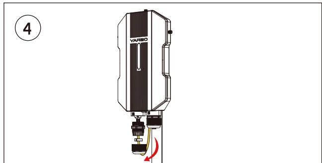
Thread the ethernet cable through the gland and its cover. Locate the opening of the black rubber plug and snap it onto the ethernet cable.
