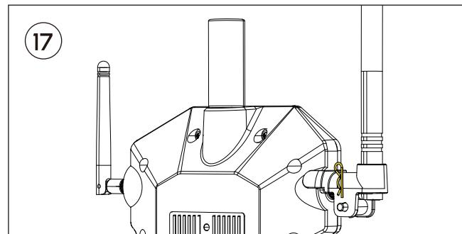
Pass the R-clip through the holes in the Clevis Pin, making sure the Clevis Pin are secure.
