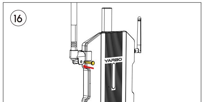
Tighten the Clevis Pin to ensure that the antenna is secure.
