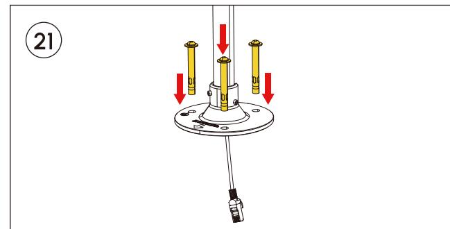
Secure the mount by fastening the three connection bolts (use wood screws for wooden surfaces, expansion bolts for hard surfaces like concrete or walls, and grass pegs for lawns).
