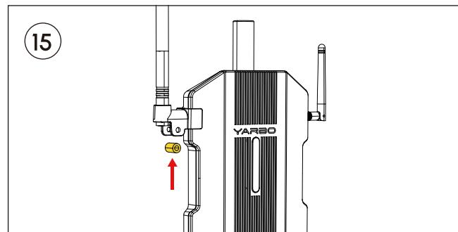
Move the Halow Antenna Clips to the bottom of the Halow Antenna and snap the Data Center. Then put on the Clip bushing.
