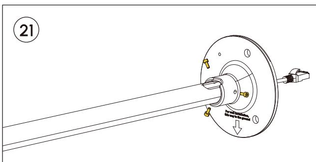
Screw in three connection bolts for pole to stabilize the mount and standard pole.
