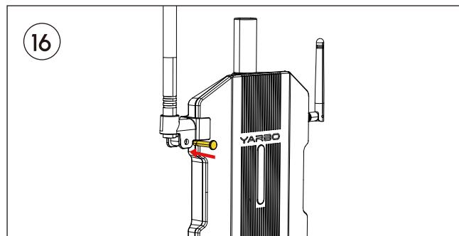
Tighten the Clevis Pin to ensure that the antenna is secure.
