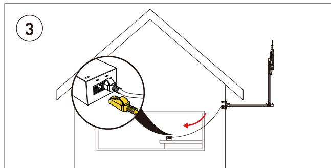
Pull the Ethernet cable that has been threaded through the Data Center Set and connect it to the POE port of the POE power adapter.
