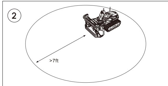
**Drive** Yarbo to the desired location for the Docking Station to test if there is strong GPS signal. Once Yarbo reaches a position with a strong GPS and network connection, the app will notify you.
