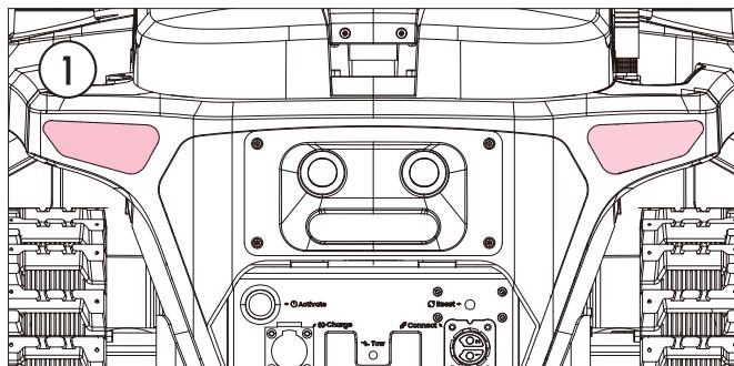
Before proceeding, ensure that Yarbo is powered on. A solid red light on the Yarbo (shown on following figure) indicates that Yarbo is powered on and ready for the controller setup.
