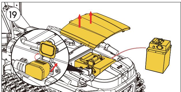
**Remove** the cover by grasping both sides with your hands and place the battery inside. **Connect** the cable from the Yarbo Core to the battery.
