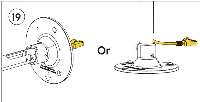
Thread the ethernet cable through the middle hole of the mount , or pull out the Ethernet cable through the opening or gap in the pole carefully.
