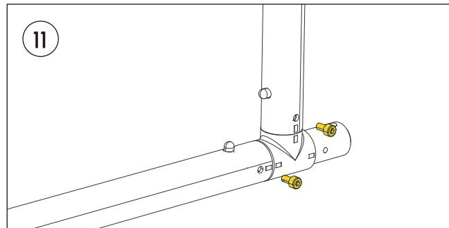
Screw in the two connection bolts to stabilize the T-joint, standard pole, and extension pole.
