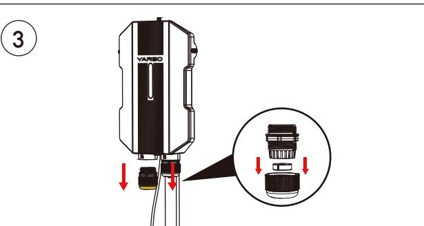
Carefully unscrew the entire gland set on the WAN port of the Data Center. Remove the gland cover and push out the black rubber plug.
