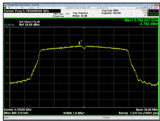
(802.11n20) PSD plot on channel 165
