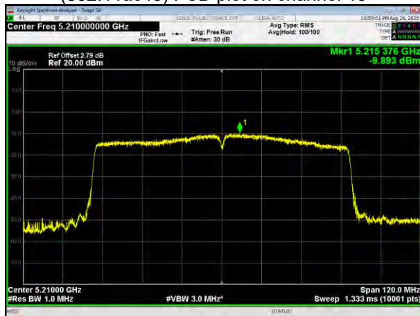
(802.11ac40) PSD plot on channel 46
