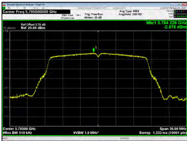
(802.11a) PSD plot on channel 165
