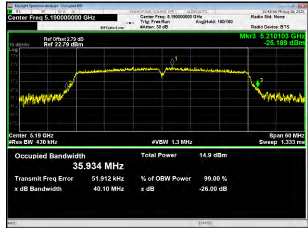
(802.11 n40) plot on channel 46
