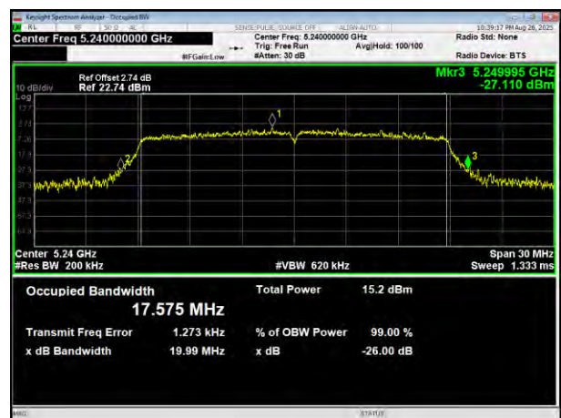
(802.11 n20) plot on channel 48
