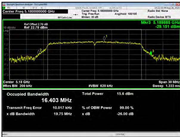
(802.11a) plot on channel 36
