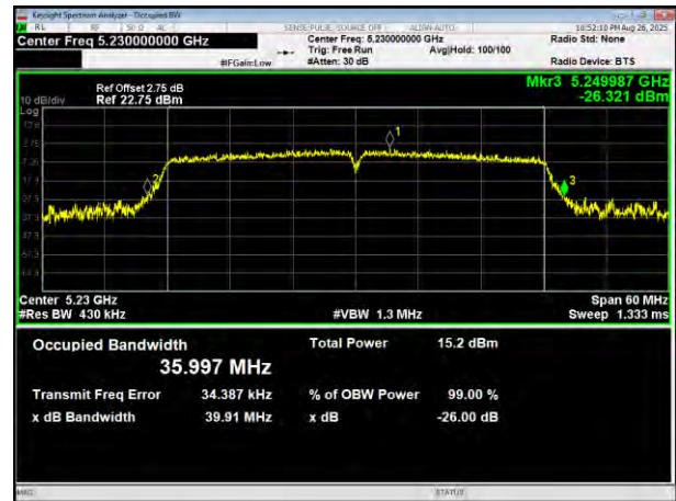
(802.11 n40) plot on channel 46
