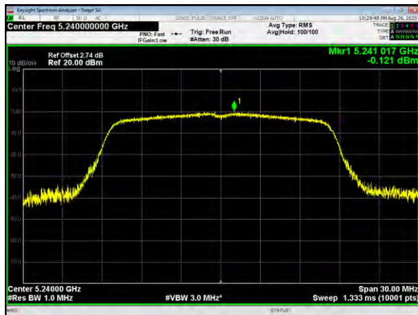
(802.11a) PSD plot on channel 48
