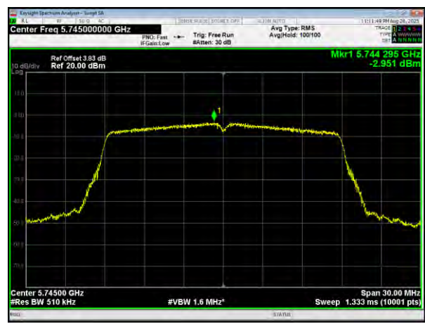
(802.11n20) PSD plot on channel 157
