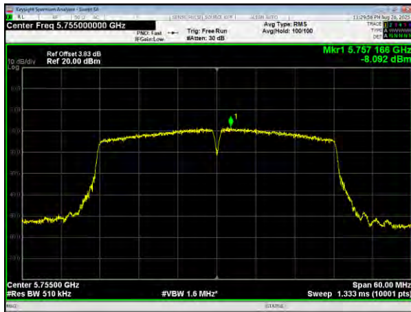
(802.11ac40) PSD plot on channel 159
