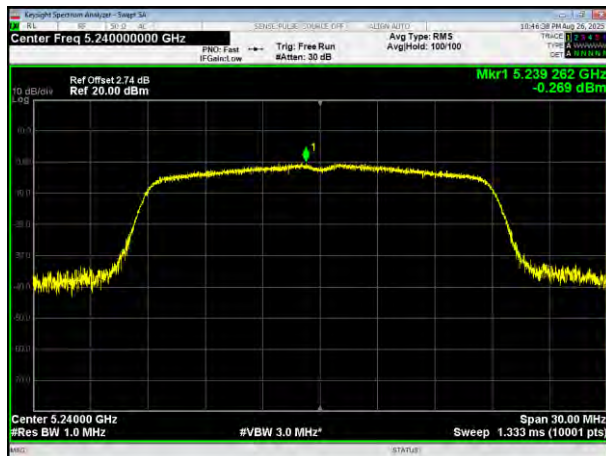
(802.11ac20) PSD plot on channel 48
