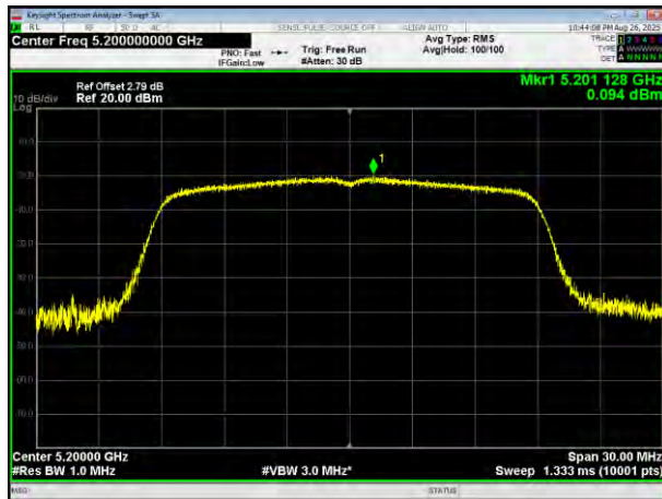
(802.11ac20) PSD plot on channel 48
