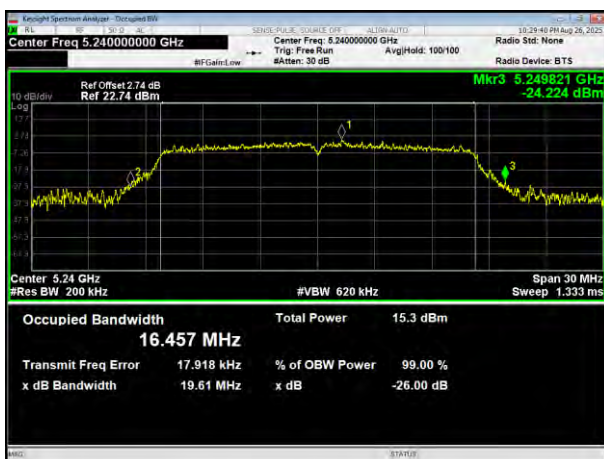
(802.11a) plot on channel 48
