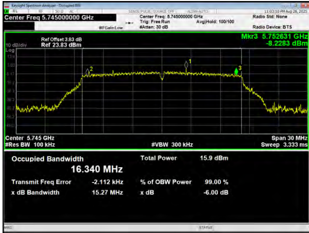
(802.11a) plot on channel 157
