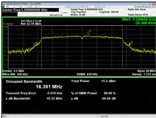
(802.11a) plot on channel 48
