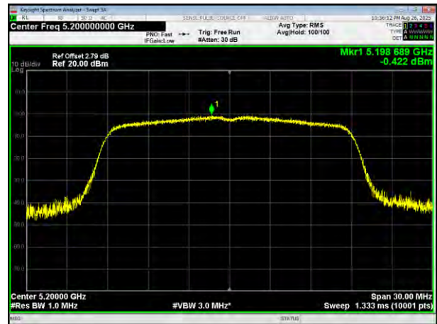
(802.11n20) PSD plot on channel 48
