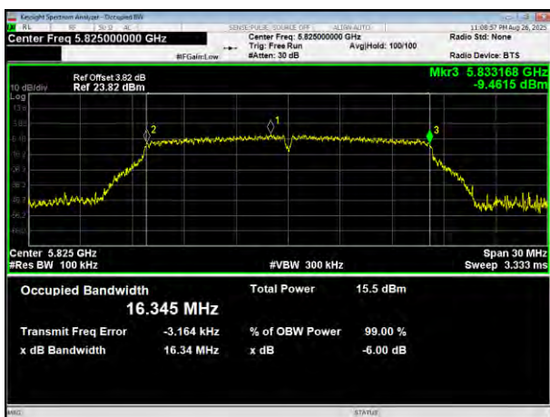
(802.11a) plot on channel 165
