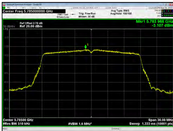
(802.11ac20) PSD plot on channel 157
