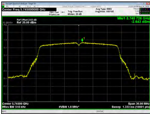
(802.11a) PSD plot on channel 157
