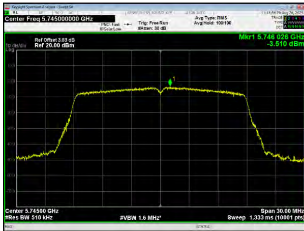
(802.11ac20) PSD plot on channel 157
