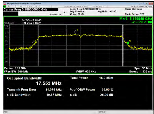
(802.11 n20) plot on channel 36
