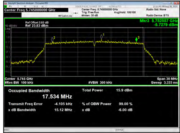
(802.11 n20) plot on channel 157
