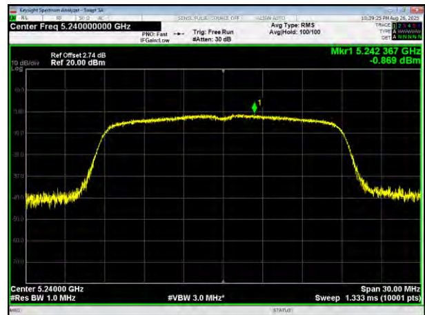
(802.11n20) PSD plot on channel 48
