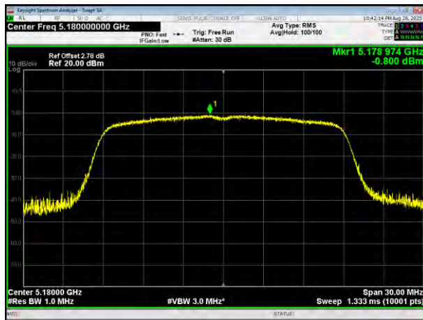
(802.11ac20) PSD plot on channel 36
