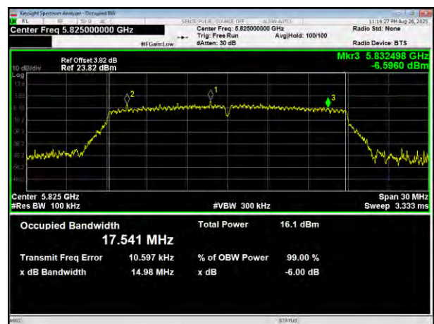
(802.11 n20) plot on channel 165
