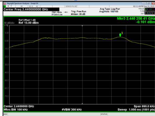
In-Band Reference Level BLE 1M_Channel 19
