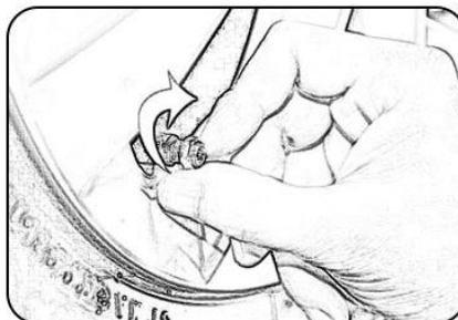
2. Tighten the anti-theft nut securely onto the tire until it is fully seated.
