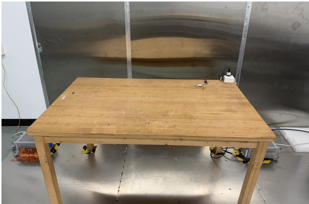
**1.2 Radiated Emission below 1GHz****30M-1GHz:**
