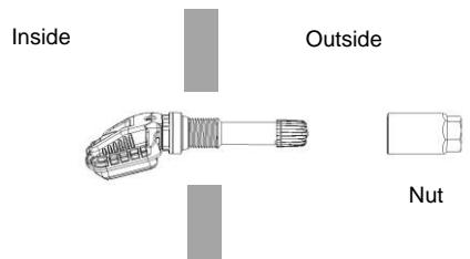
1.4 Place nut on the valve stem, and tighten with 5 Nm (44 inch pounds) torque.
