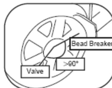
2.2 Firmly fix the wheel on the turntable clamps. (If the mounting head of the tyre changer is positioned at 12 o'clock, then the valves stem should be at the 11 o'clock position.) Apply lubricant to both tyre bead and rim, and then remove the upper tyre bead.
